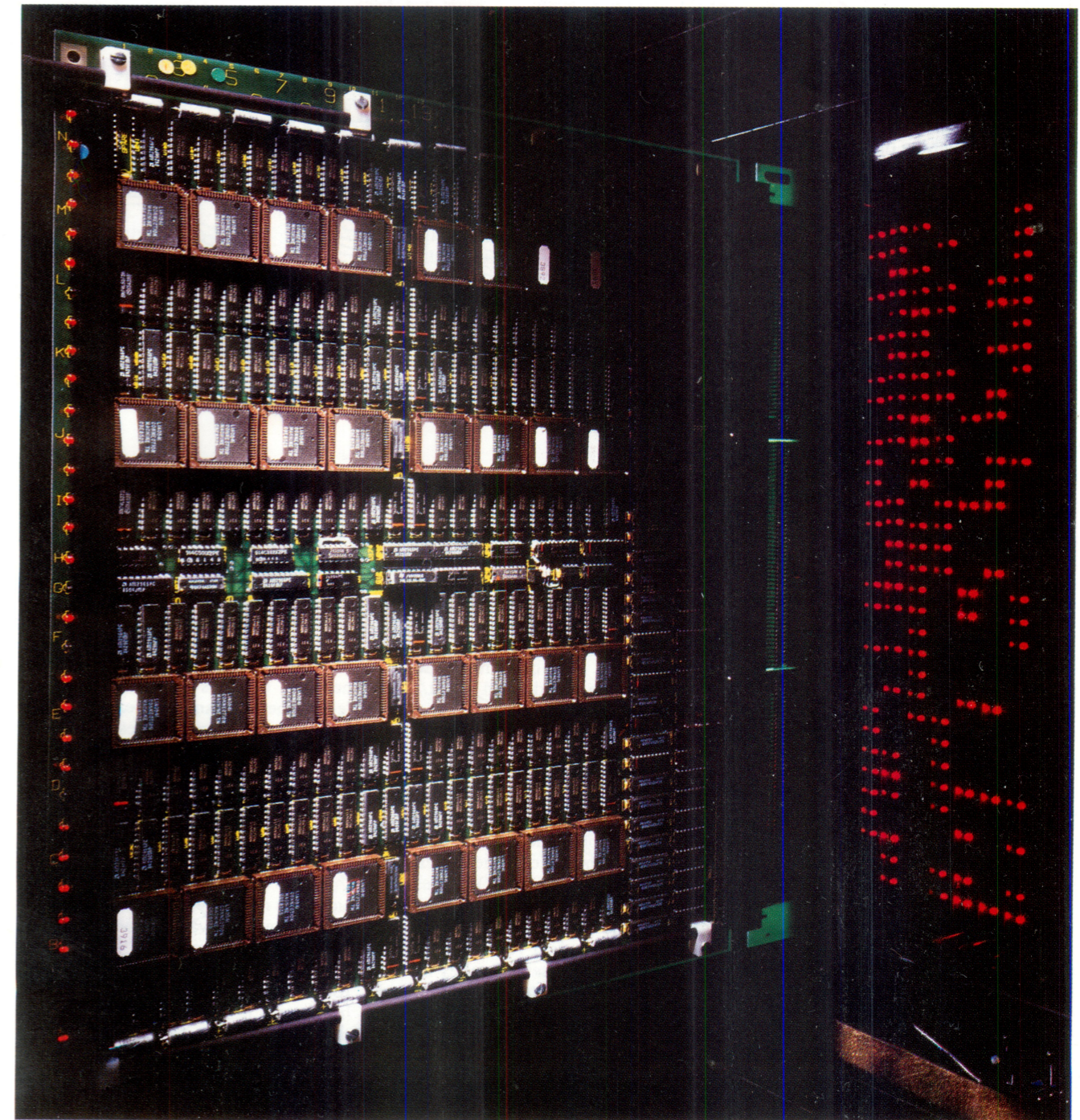
BOARD slides out of the Connection Machine much like a book from a shelf. The square objects are the chips, each with its 16
